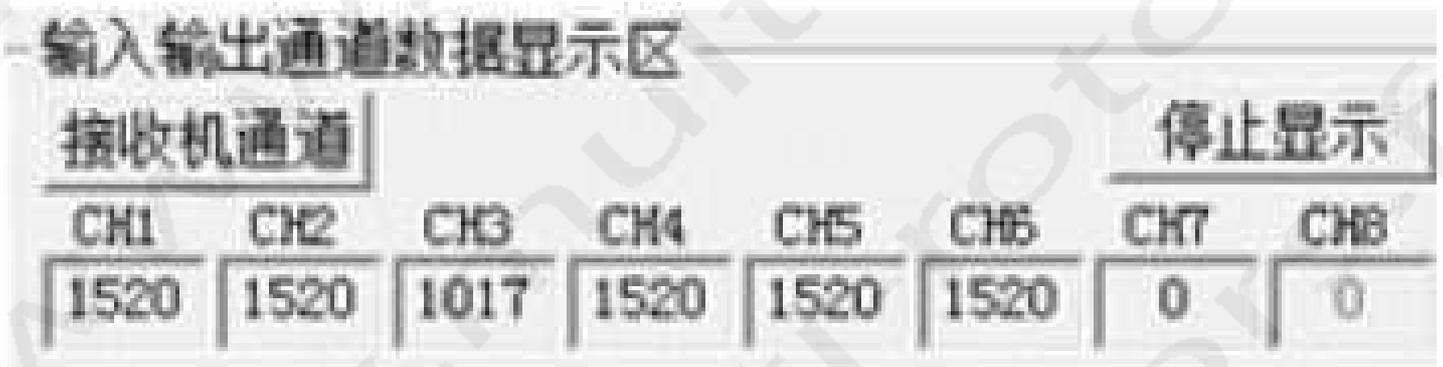
The screenshot shows a software window titled "输入输出通道数据显示区" (Input/Output Channel Data Display Area). It features a table with 8 columns labeled CH1 through CH8. The first column is labeled "接收机通道" (Receiver Channel) and the last column is labeled "停止显示" (Stop Display). The data values are: CH1: 1520, CH2: 1520, CH3: 1017, CH4: 1520, CH5: 1520, CH6: 1520, CH7: 0, CH8: 0.
